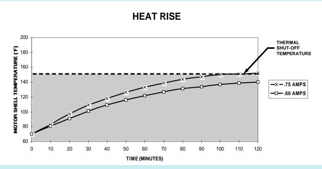
The shaded area in both the Performance Data and Heat Rise charts, contains pumps with current levels that are capable of running without periodic cool down. Pumps in this category will generally transfer more water over sustained periods than those in the unshaded areas, which are required to shut down while the motor cools. Some applications require maximum flows at high pressures for relatively short periods, however, so an explanation of thermal protection follows:
